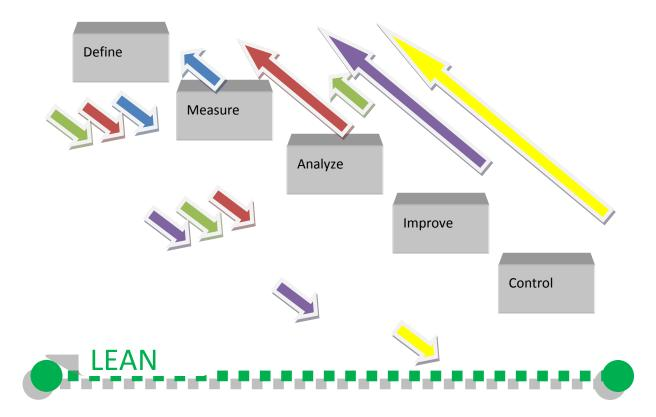
This diagram is intended to track the cycles of the process. Each color represents a cycle. As the project was finally defined, the iteration continued as new information was discovered during subsequent phases. Lean methodologies were applied throughout, but it drawn here to also express the impact on the DMAIC process.
